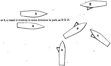
If A sees a White Mast-head Light above the Red Light, A knows that the vessel is a steam-vessel, and is either approaching her in the same direction, as B, or is crossing to port in some direction, as D D D.
