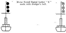
Directions.—A dredger showing this signal must not be passed until the position is made clear by the exhibition of a Passing Signal.
