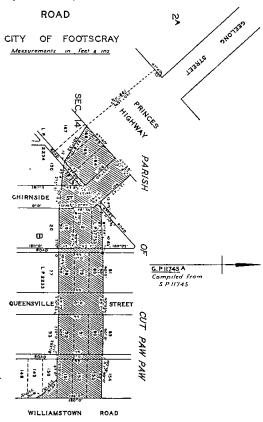
The land shown hatched on plan numbered G.P.117458 hereunder required for the widening of Geelong-street in the City of Footscray and making of the widening thereon.
