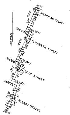
The land shown hatched and crosshatched was on the 25 · 7 · 1969 contained in CIT 1677 · 365 Measurements are in links
