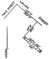
The fee of the road shown hatched was contained in CIT 2509-670 on the 23.7.1969. Measurements are infect & inches.
