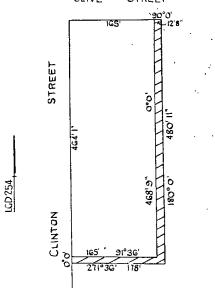
The road shown hatched was on the 24 .7 1969 contained in CIT 4419-662. Measurements are in feet and inches.
