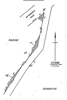
The land shown hatched on Plan numbered G.P.12293 hereunder, required for the widening of the Frankston-Flinders road in the Shire of Hastings and making of the widening thereon.
