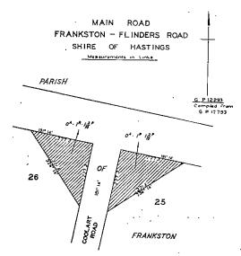
The land shown hatched on Plan numbered G.P.12294 hereunder, required for the widening of the Bittern-Dromana road in the Shire of Hastings and making of the widening thereon.
