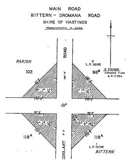
The land shown hatched on Plan numbered G.P.12295 hereunder, required for the widening of the Mornington-Tyabb road in the Shire of Hastings and making of the widening thereon.
