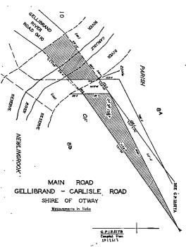
The land shown hatched on Plan numbered G.P.12517c hereunder required for the deviation from the Gellibrand River-road in the Shire of Otway and making of the deviation thereon.
