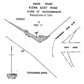
The land shown hatched on Plan numbered G.P.12688b hereunder required for the widening of Gundowring-road in the Shire of Yackandandah and making of the widening thereon.
