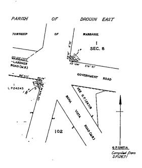
The land shown hatched on Plan numbered G.P.12671s hereunder required for the widening of Bona Vista-road in the Shire of Warragul and making of the widening thereon.
