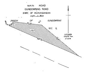
The land shown hatched on plan numbered G.P.13369 hereunder required for the widening of Gundowring-road in the Shire of Yackandandah and making of the widening thereon.
