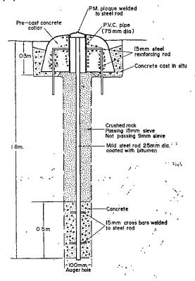
Combined P.M. and Bench Mark. Concrete collar can move up or down with surface movement whilst the plaque and rod remain stable
