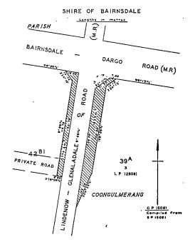
The land shown hatched on plan numbered G.P.15002a hereunder required for the widening of Buckland Valley Road in the Shire of Bairnsdale and making of the widening thereon.
