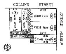
AREA OF RIGHT OF WAY SHOWN HATCHED HAS BEEN CLOSED AREA OF RIGHT OF WAY SHOWN CROSSHATCHED IS TO BE CLOSED & SOLD TO ABUTTING OWNERS UNDER SECTION 528(2) OF THE LOCAL GOVERNMENT ACT PROVIDED STORMWATER & SEVERAGE EASSMENT RIGHTS ARE MAINTAINED.
