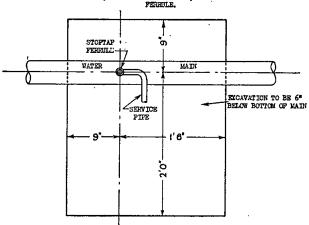
FOR LARGER MAINS OR FOR THOSE LAID DEEPER THAN SHOWN ABOVE, THE DIMENSIONS SHALL BE INCREASED.
