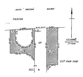
The land shown hatched on Plan numbered G.P.11681 hereunder required for the widening of the Coleraine-Edenhope road in the Shire of Kowree and making of the widening thereon.
