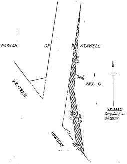
The land shown hatched on Plan numbered G.P.12608 hereunder required for the widening of the Stawell-Warracknabeal road in the Shire of Stawell and making of the widening thereon.
