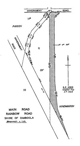
The land shown hatched on Plan numbered G.P.12635 hereunder required for the deviation from Rainbow-road in the Shire of Dimboola and making of the deviation thereon.
