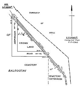
The land shown hatched on plan numbered G.P.13303 hereunder required for the widening of Jumbuk-road in the Shire of Morwell and making of the widening thereon.
