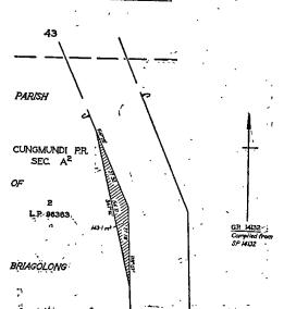
The land shown hatched on plan numbered G.P.14036 hereunder required for the deviation from the Yarram-Traraigon road in the Shire of Rosedale and making of the deviation thereon.
