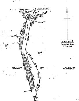
The land shown hatched on plan numbered G.P.14505 hereunder required for the deviation from Tarwin Lower Road in the Shire of Woorayl and making of the deviation thereon.
