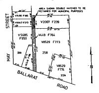
AREA OF RIGHT OF WAY SHOWN HATCHED IS TO BE CLOSED & SOLD TO ABUTTING OWNERS UNDER SECTION 528(2) OF THE LOCAL GOVERNMENT ACT PROVIDED STORMWATER & SEWERAGE EASEMENTS ARE MAINTAINED
